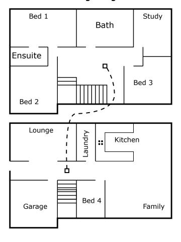
Use of the wired interconnection between levels ensures alarm signalling even if floors are of heavyweight construction.
